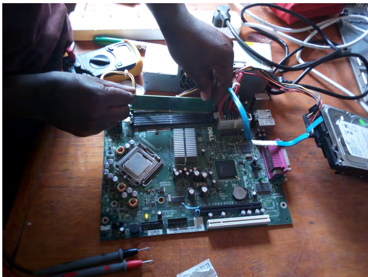
Technician replacing RAM
